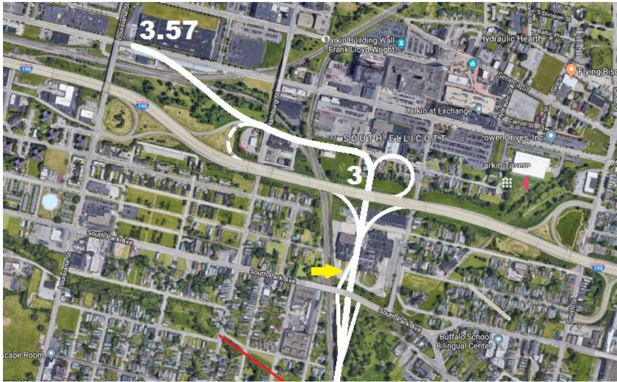
Fig. 16: The yellow arrow points to a possible additional “escape” offramp to South Park Avenue – but the crossover merge zone between this possible offramp and the onramp from I-190 may be unduly short.
